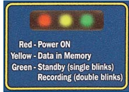
LED s indicate mode of operation
