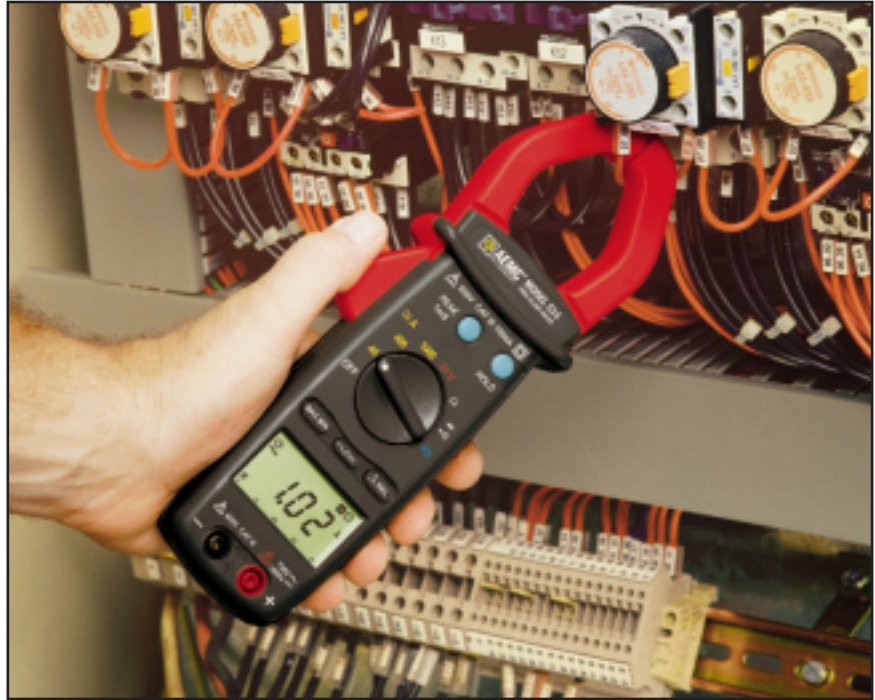
Model 514 measuring primary current on a machine control system.
