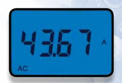
2. Start **True ImRush** acquisition. The clamp then displays the trigger threshold and begins the monitoring phase.
