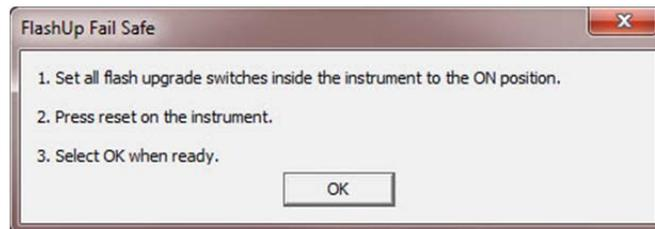
**Step 6:** To access the flash upgrade switches when performing a fail-safe upgrade, the instrument must be removed from the case. The upgrade switches and reset switch are located on the main pcb under the TEST button.
