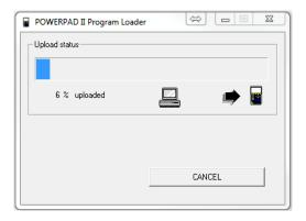
**Step 10**: The instrument will automatically turn off when the firmware is loaded and the memory is erased. The window below will appear if successful. Upgrade should only take a few minutes.
