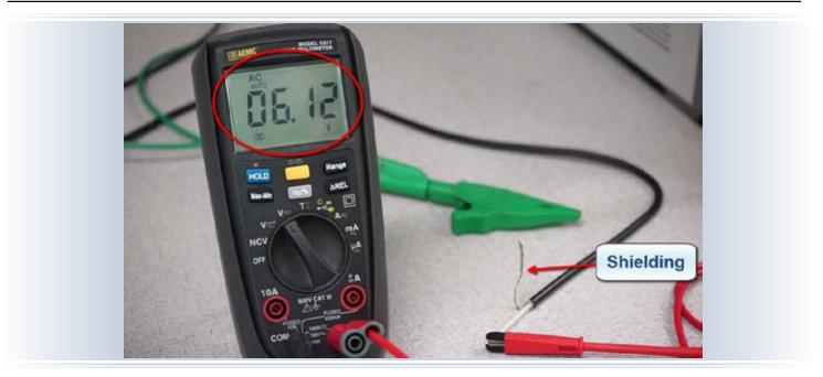
As you can see, the noise voltage being generated within the cable is over 6V, a voltage that could potentially corrupt data sent through the cable.
