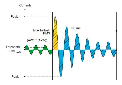
AEMC provides power clamp-on meters that provide True InRush capability. These instruments feature high-speed, digital signal processing to filter out electrical noise and capture inrush current to a high level of precision and repeatability. They include the 400 Series and 600 Series families of clamp-on meters. AEMC also offers other 3 phase analyzers, including the Model 8333 and Model 8336, that provide True InRush detection and storage.
