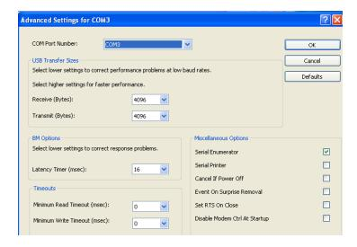
4. Launch the Simple Logger software and select the COM port from the Port menu.
