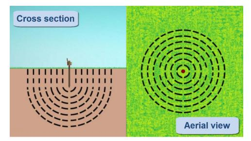
Grounding systems can range in complexity from a single rod driven into the ground, to complex grids consisting of multiple rods connected with wire mesh, to other types of grounding systems incorporating plates, concrete, chemicals, and soil conductivity enhancers.
