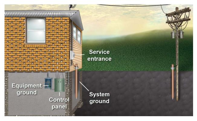
The system ground can be a simple metal rod driven into the ground as shown above, a grid consisting of multiple electrodes, or another type of grounding system.
