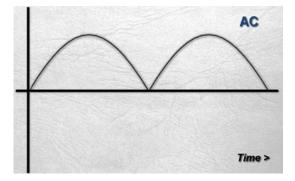
As you can see, all points on the graph are at or above zero, so we no longer have to deal with negative values. We can now use these positive numbers to calculate the effective power of this AC system. A step-by-step derivation of these calculations requires a moderate amount of math; so for the sake of brevity we'll cut to the chase and show the final formula, which for sinusoidal voltage is as follows:
