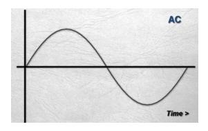
If we measure the voltage or current at random times on this graph, we get different values, depending on which points we choose. At first glance, it may seem logical to simply take the average of these measurements to calculate the effective power for this source. However, if we do so, we'd end up with a voltage or current of zero. By definition, the pure sinusoidal AC power wave cycle spends as much time below zero as above, therefore the negative values will cancel out the positive ones.
