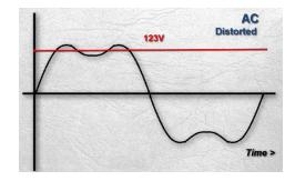
In other words, the harmonic distortion introduced in the waveform shown above has changed the V<sub>RMS</sub> from 120V in its pure sinusoidal form to approximately 123V in its distorted form.
