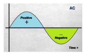
So no matter how high our peak power is, the average power for the classic AC system would always be zero, the same as if we had no power source at all. Obviously such a result tells us nothing about the true power flow in this system, so we need another way to derive the effective AC voltage or current.
