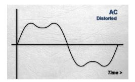
As you can see, the greatest distortion to the fundamental occurs when the 3rd harmonic reaches either its positive or negative peak. By definition, this occurs 6 times per cycle of the fundamental. Therefore to accommodate the effect of the 3rd harmonic, we will take 6 measurements, timed to correspond with the positive and negative peaks of the third harmonic:
