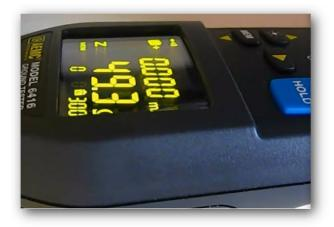
The OLED display is also ideal for bright ambient conditions. For example, when viewing outdoors in sunny conditions, press the brightness + button on the instrument's front panel to enhance the contrast on the screen. With the display contrast set to high the screen is now easily visible even in the brightest natural conditions.
