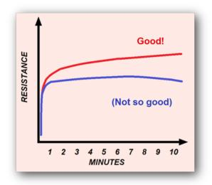
When you plot the results, you should see a curve that rises relatively rapidly at first, and then continues to gradually rise throughout the testing period. If instead the curve is relatively flat or begins to turn down as the test progresses, moisture, dirt, or other factors may be compromising your insulation.
