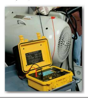
To assess and monitor insulation integrity, several tests have been developed. These typically involve injecting a test voltage and then measuring resistance. This "stress tests" the insulation, similar to applying high water pressure to plumbing to test for leaks.
