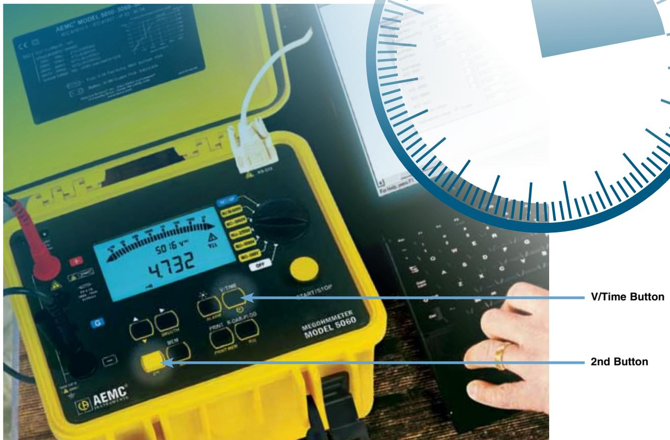
**Figure 1.** Front panel buttons used to activate a timed recording
