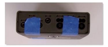
**3.** Turn over the PEL, and locate the six fastening screws on the back of the instrument.
