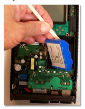
**8.** Inspect the plug of the replacement battery pack, and note the position of the connector pins (see below).
