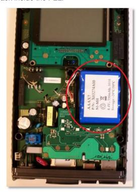
**7.** Gently remove and unplug the battery from the PEL. A small non-conductive implement such as a drink stirring stick (shown below) can be useful for doing this.
