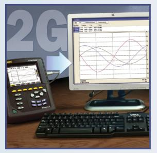
The 8335 is capable of downloading up to 2 Gigabytes of data for Trend Reports. This has the ability to represent each recording parameter measured every second for a month. The download time for this much memory usage would be approximately 14 hours. Time, sample rate, number of measured parameters, and the kind of parameter would determine how much memory is required.
