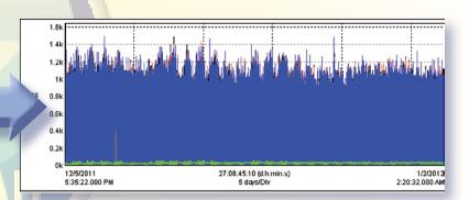
Some hints that the entire report is not fully downloaded are found in looking at the graph. A long report would turn the graph almost solid and the time at the bottom would not reflect the sample rate selected in the initial set up of the recording.
