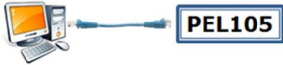
Point-to-Point Ethernet communication establishes a direct link between the computer and the instrument via Ethernet cable. To do this, you must be connected to the instrument via a USB connection ([Lesson 1](#)). Then proceed as follows:
