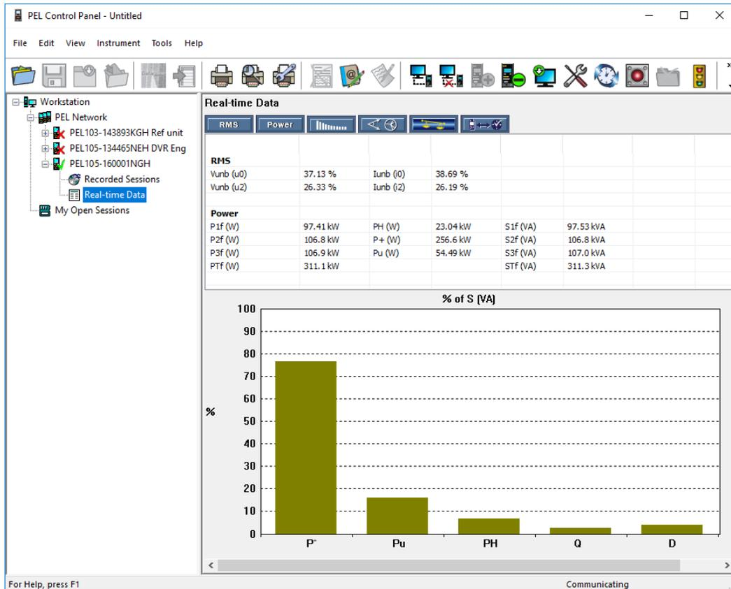
At the top of the frame is a table displaying a variety of parameters. The first four are unbalance values:
