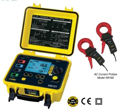
The Ground Resistance Tester Model 6471 is a portable measurement instrument designed to measure Ground Resistance with 2 clamps (no auxiliary rods), Bond/Connection Resistance (2-Pole and 4-Pole Kelvin sensing). Ground Resistance (3-Pole or 4-Pole), Ground Coupling Resistance, and Selective Ground Resistance, Soil Resistivity (Wenner or Schlumberger method).
