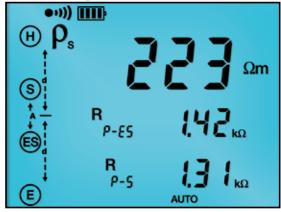
The Schlumberger test displays test lead connection, soil resistivity (p) test results, test electrode resistance and more.
