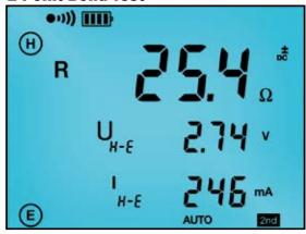
The 2-Point Bond test displays lead connections, bond resistance test results, test voltage and current.
