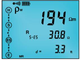
The Wenner test displays test lead connection, soil resistivity (p) test results, electrode spacing and resistance.
