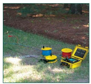
The Model 6472 performs an automated way to measure the value of the earth/ground using the Fall-of-Potential method and storing measurements.
