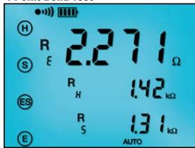
The 4-Point Bond test displays lead connections, bond resistance test results, test voltage and current.
