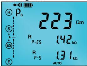
The Schlumberger test displays test lead connection, soil resistivity (p) test results, test electrode resistance and more.
