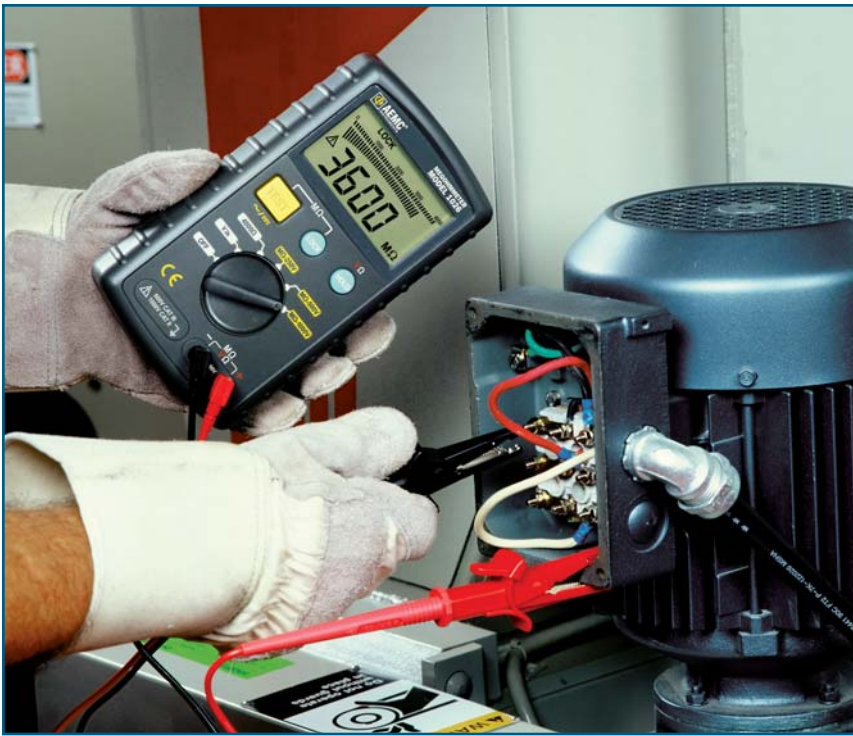
Model 1026 quickly verifies the isolation of all the connections in the box.
