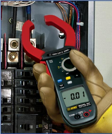
The TRMS Clamp-On Meter Models 400 & 600 Series provide a new standard for safety and measurement capability not available in any other clamp meter sold today. Safety rated at 1000V CAT IV, they are safe to operate in all electrical environments. They are rugged enough for the most demanding work environments and will withstand both dust and water spray with their IP54 rating. They are ergonomically designed and easily used by one hand, including function
