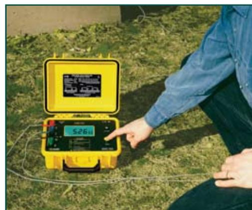
Model 4630 testing ground rod of a pad-mount transformer.
