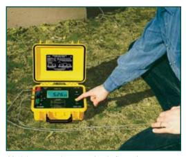
Model 4630 testing ground rod of a pad-mount transformer.
