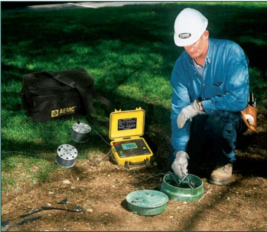
Model 4630 performing a 3-Point ground resistance test on an individual rod.
