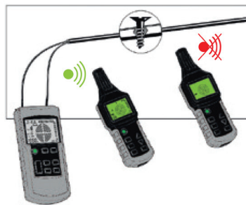
Short circuit detection in walls, flooring or under ground
