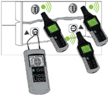
Location and tracking of branches and outlets
