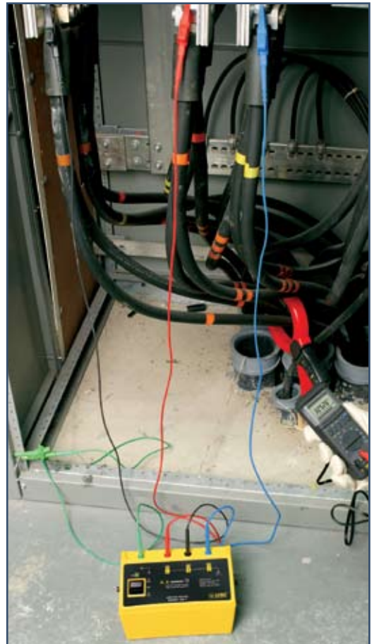
Model AN-1 creates a momentary ground to assist in fault current detection.
