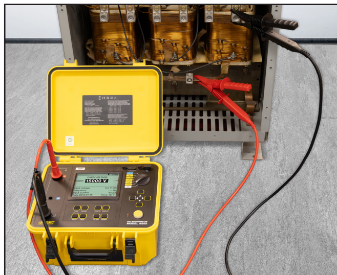
Model 6555 performing a single-phase test on a three-phase transformer.
