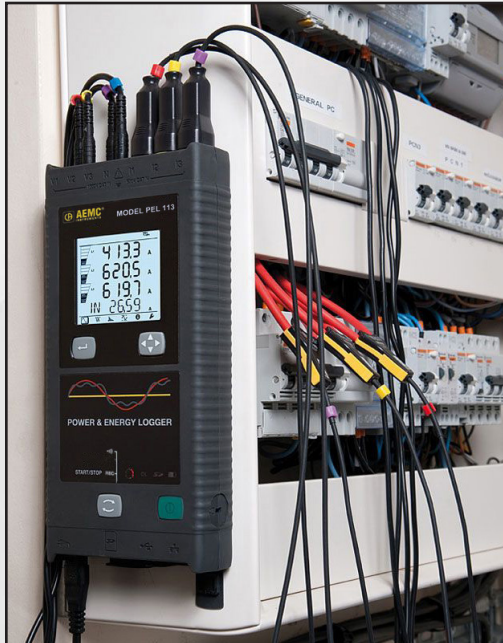
Models PEL 112 and PEL 113 are equipped with powerful magnets for mounting.
