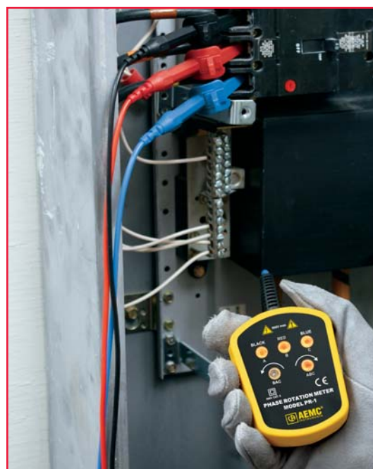
Model PR-1 quickly identifies proper phase sequence in an industrial panel
