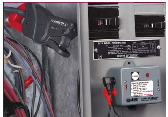
Model L110 with 200A AC Current Probe Model MN213
