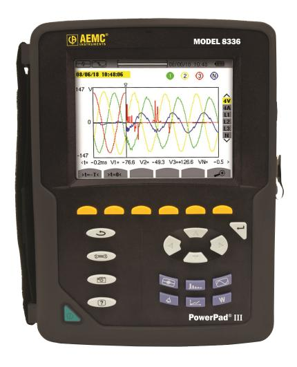
The PowerPad can detect and record short-term anomalies such as transients and inrush current. You can also configure alarms to identify when a measurement falls outside defined parameters. The PowerPad takes 256 samples per cycle, resulting in over 15 thousand samples per second on 60Hz networks. This allows the instrument to calculate highly detailed sub-cycle data. PowerPad can also measure neutral voltage and current, and supports 5-wire networks.
