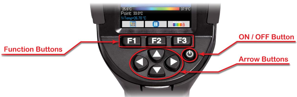
Press the F1 button to display the Main configuration screen. Then use the arrow keys to highlight the Parameter icon, and press F2. This displays the Parameters screen.
