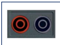
Jacks: Two standard safety banana jacks (4mm)
