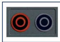
Jacks: Two standard safety banana jacks (4mm)
