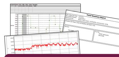
Reports can be displayed on a PC and printed. Each report includes all test results in a tabular and graphic format, as well as operator and test site information.
