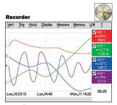
The OX<sup>III</sup> Series supports a great variety of sensors (voltage, current, temperature, 0 to 10V, 4 to 20mA, etc) and displays them in their original physical scale and units.
