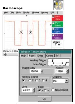
Triggering menu allows selection of type, duration, delay, count and more using touch screen drop-down menu.
