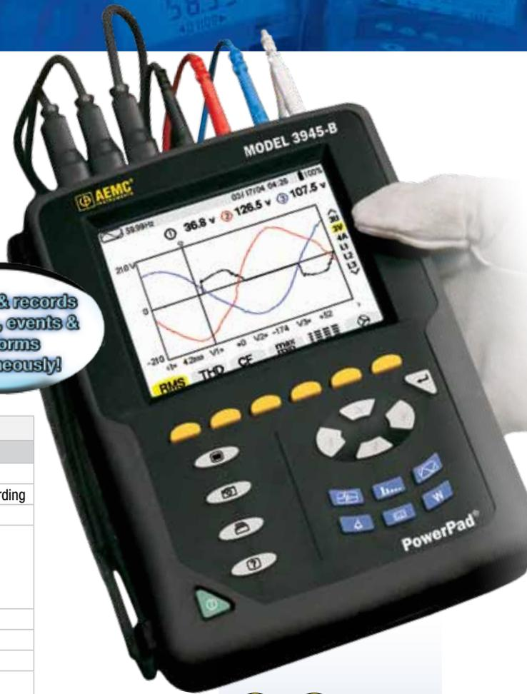
Three voltage and three current inputs
