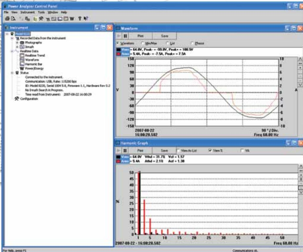
DataView® software provides a convenient way to configure and display power quality measurements from your computer. Through the use of clear and easy-to-use tabbed dialog boxes, all PowerPad® functions can be configured and tests can be initiated. Results can be displayed in real-time and stored in your PC. Reports may be printed along with the operator's comments and analysis.
