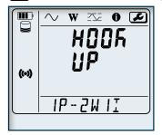
Hook up, Wi-Fi, aggregation period, can be configured from the front panel of the PEL 52. Current ratios and number of turns need to be configured via the PEL Transer software based on the current sensor type.
