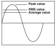
Figure 9. RMS — Avg — Peak Relationship in sine wave
