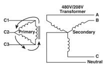
Figure 7. Delta primary, circulating current
