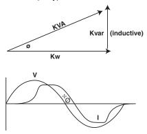
Figure 4. Power factor on nondistorted sine wave.
