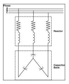
Figure 10. Single tuned shunt filter.
