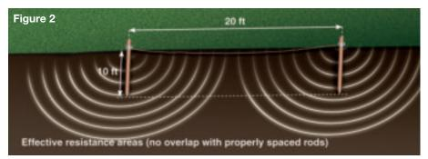
multiple 10 foot rods should be spaced 20 feet apart to avoid being in the sphere of influence of each other (See figure 2).
