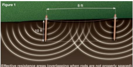
Effective resistance areas (overlapping when rods are not properly spaced)
