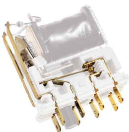
POK relay with gold-plated contacts and terminals plus tropicalized coil.
