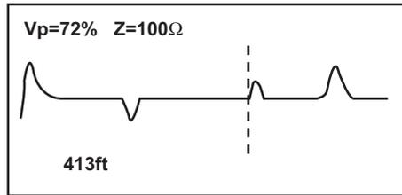
On the fault curve shown in the previous two screens, a low impedance event occurs at 210 ft, shown by a downward spike on the curve, and a high impedance event occurs at 413 ft.
