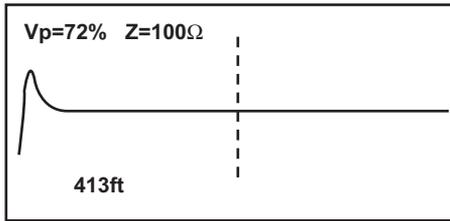
The following display shows a cable with impedance anomalies on it.
