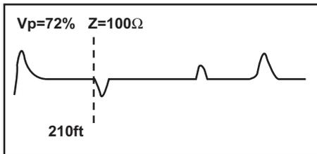
The vertical cursor line is moved left and right along the line of the trace by pressing the ◀ and ▶ buttons.
