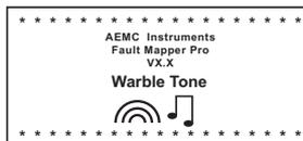
The injected signal oscillates between 810 and 1110Hz, six times per second.
