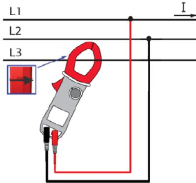
**NOTE:** 3-phase power on a balanced 4-wire network can also be measured by proceeding in the same way, or by proceeding as for the measurement on a single-phase network, then multiplying the value by three.
