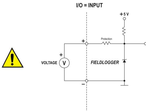
Fig. 14 - Voltage connection
