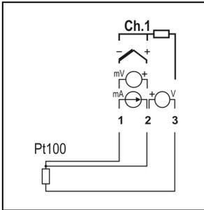
The RTD connection for the channels is made to the terminals in accordance with the figure at the left. The 3-wire connection from the Pt100 sensing element to the **Data Logger** input guarantees the cancellation of the error caused by the lead resistance. All three wires must have the same gauge and length.
