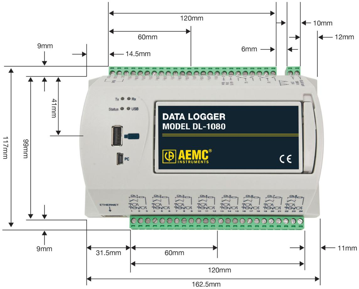
**Fig. 04** – Dimensions without DISPLAY module
