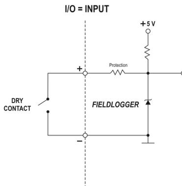
Fig. 15 - Dry-contact connection
