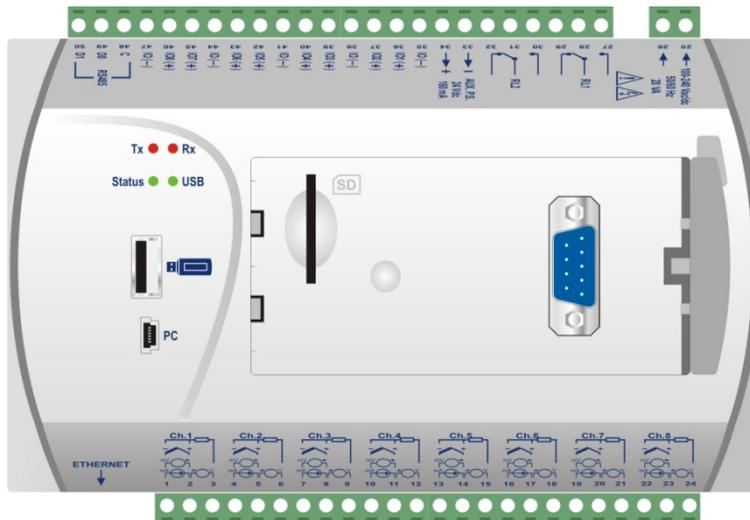
**Fig. 20 - Data Logger connectivity resources**
