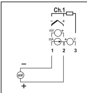
The millivolt connection for the channels is made to the terminals in accordance with the figure at the left. Please observe the correct polarity of the connection.
