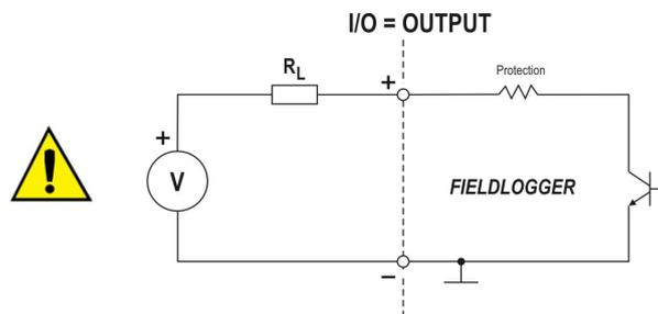
Fig. 17 - Connection of a load  $R_L$  to a digital output
