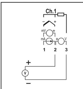
The voltage connection for the channels is made to the terminals in accordance with the figure at the left. Please observe the correct polarity of the connection.
