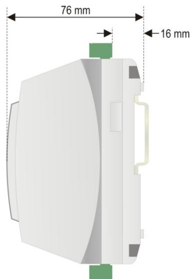
**Fig. 06** – Dimensions of the side with DISPLAY module
