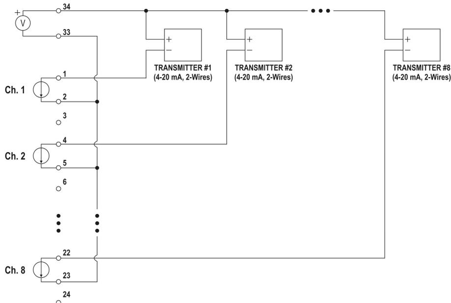
Fig. 19 – Auxiliary power supply powering 4-20mA (2-wire) transmitters
