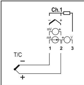
The Thermocouple connection for the channels is made to the terminals in accordance with the figure at the left. Please observe the correct connection polarity.
