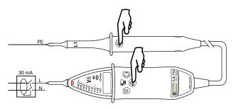
If the voltage measured is between 8 Vrms and 400 Vrms, the test is triggered.
