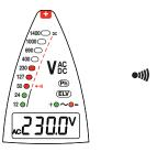
■ DC: the indicators light up to indicate its value, and the + (green) indicator or the - (orange) indicator lights up to indicate the polarity.
