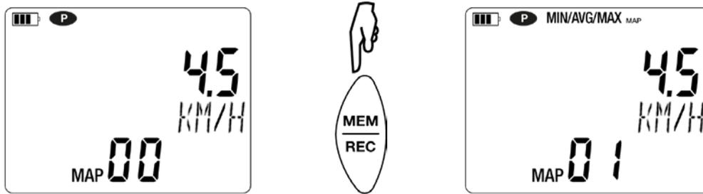
When all points have been measured, you can display the maximum, average, and minimum values. To do this, press  $\frac{\text{MAX}}{\text{AVG}}/\text{MIN}$  three times to cycle through the maximum, average, and minimum values respectively.
