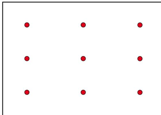
To enter MAP mode, press <sup>°C / °F</sup> <sub>MAP</sub> for >2 seconds. Place the sensor at the first measurement point and press <sup>MEM</sup> <sub>REC</sub> to record the value in memory. The MAP counter is incremented. Repeat this step for all the other points of the map.
