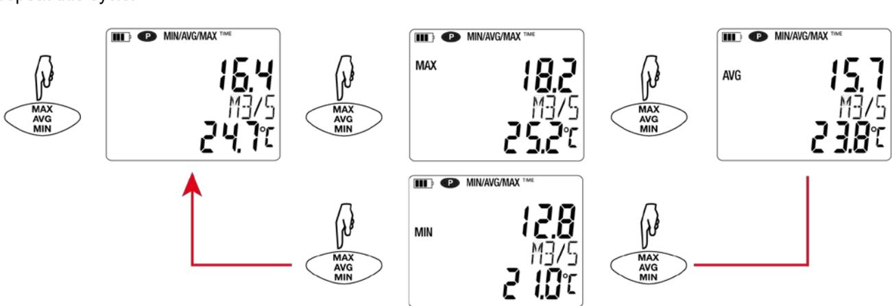
To exit MAX AVG MIN mode, long-press <sup>MAX
