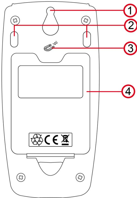
1. "Tear-drop" notch to hang instrument
