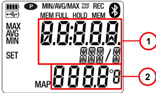
1. Air speed and flow display measurement
