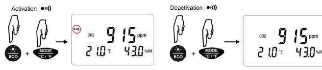
First press the **ECO** key, then, while keeping it pressed, press the **MODE** key.
