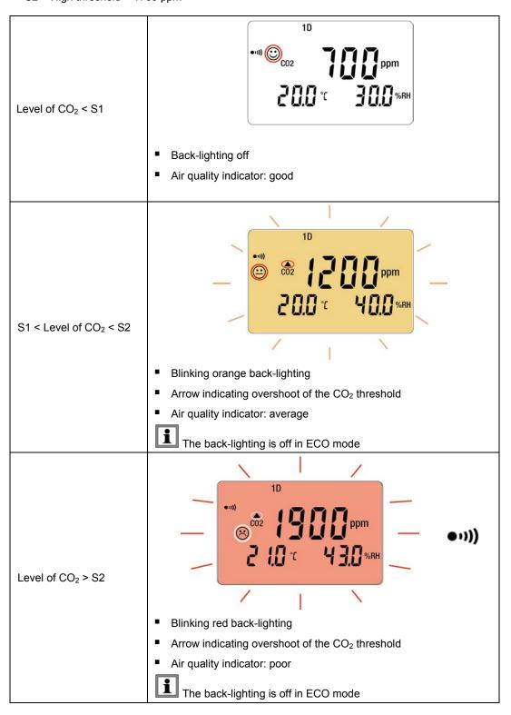
**3D mode:** Activation of the visual (and, if activated, audible) warnings during overshoots of the temperature, humidity, and/or CO<sub>2</sub> comfort zones.
