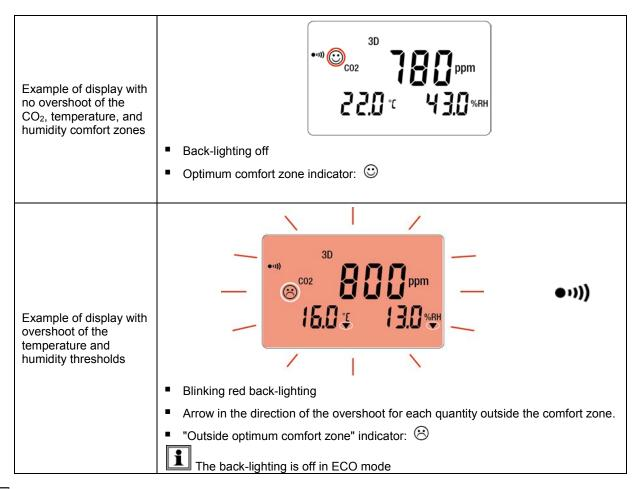
For the **1D** and **3D** modes, if the buzzer is active, it will sound intermittently upon the appearance of the experimental symbol.
