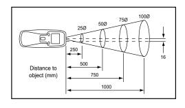
surroundings. Remember that the measurement size is one-tenth the distance to the target. For example, if the thermometer is at 10", then the size measured is 1".
