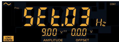
if file 3 contains a configuration the data (except frequency) is displayed on the screen.
