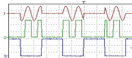
Channel 1: Main Out (sine, 1 kHz, 10 Vpp)
