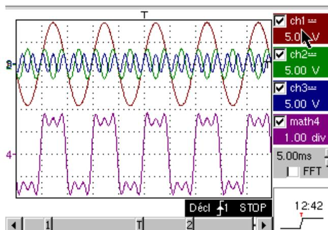
A square signal forms: the higher the number of odd harmonics the better the signal quality obtained.
