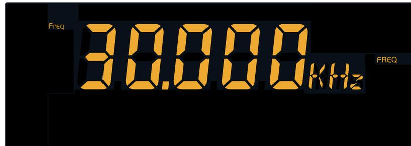
The frequency meter can measure frequencies from 5 Hz to 100 MHz with the following precision:
