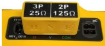
2. Observe the reading. This should be 125 $\Omega \pm 2.7\Omega$ .
