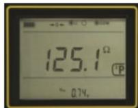
3. Press **TEST**. After a few moments the reading appears. This should be 25 $\Omega \pm 0.35\Omega$ .
