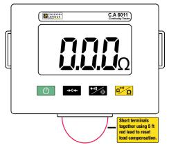
Then, from **Continuity Mode**, perform lead compensation again. This will allow for an accurate resistance measurement to be taken.
