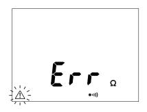
If during a continuity, resistance, or capacitance measurement the instrument detects an external voltage in excess of 15V (AC or DC), it interrupts the measurement and displays the screen show to the left.
