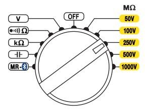
2. Use the leads to connect the system to be tested to the instrument's terminals. The system under test must be powered down and discharged. When testing insulation, the typical connection is negative (black) lead to conductor and positive (red) lead to ground or the outer insulation of the device under test.
