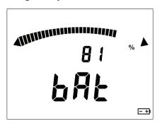
If the battery voltage is too low to ensure correct operation of the instrument, a "low battery" message appears on the LCD and the symbol blinks:
