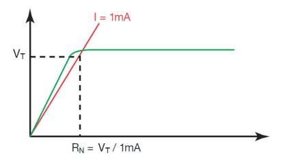
The range of operation per IEC 61557 is from  $100k\Omega$  to  $2G\Omega$  (see § 3.4).
