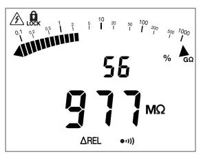
For insulation measurements, only the digital display is modified by  $\triangle REL$ . The bar graph continues to display the true measured value.
