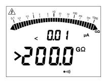
If during an insulation measurement the value to be measured exceeds the measurement range (which depends on the instrument and the test voltage), the instrument reports this condition. For example, the screen to the left is displayed when the range is exceeded on the Model 6532 while measuring in the 100V range.
