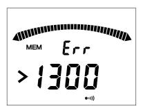
When the memory is full, the instrument displays the screen shown to the left. You must remove one or more recordings before new recordings can be saved (see § 2.3.3).
