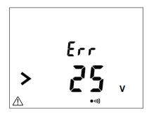
Before taking an insulation measurement, the instrument measures voltage on the system under test. If it detects voltage in excess of 25V and you attempt to take a measurement, the instrument displays the message shown to the left, and no measurement is taken.
