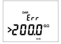
With the Models 6526 and 6532, if this condition occurs during a DAR or PI measurement, the instrument interrupts the measurement and displays the screen shown to the left.
