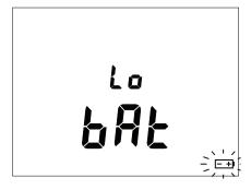
This indicates the batteries must be replaced. All batteries must be replaced at the same time. To do this:
