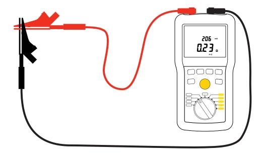
The display changes to zero and the  $\rightarrow 0$  symbol is displayed. The resistance of the leads will be systematically subtracted from all continuity measurements. If the resistance of the leads is >10 $\Omega$ , there is no compensation. The compensation remains in memory until the instrument is turned OFF.
