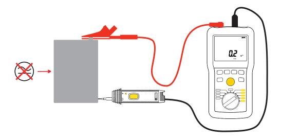
When the probe is connected, the - symbol is displayed on the instrument's LCD.
