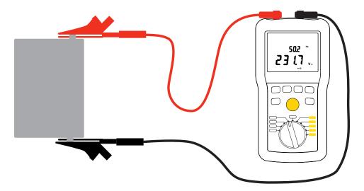
The instrument displays the voltage on the terminals. It detects whether the voltage is AC or DC; and (for Models 6526 and 6532) if it is AC, displays its frequency.
