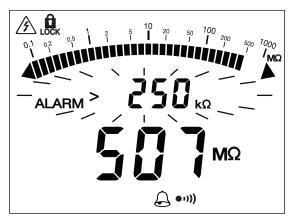
When checking continuity, this enables you to determine whether or not the continuity measurement is less than  $2\Omega$  simply by listening, without looking at the display. You can similarly check insulation quality.
