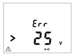
If the voltage is >15V, continuity, resistance, and capacitance measurements are prohibited.
