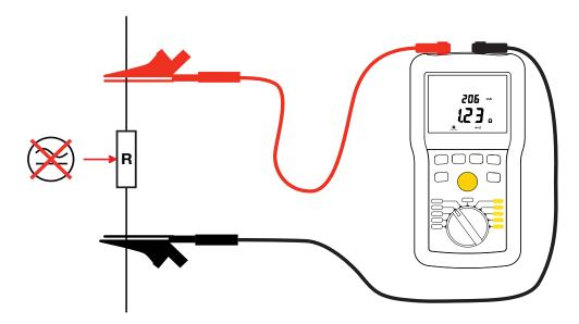
The instrument displays the resistance and the current used in the test.
