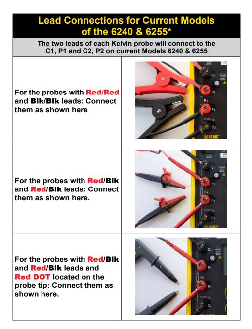
\*For Models 6240 and 6255 instruments with serial numbers lower than 1166339SEDV, terminals C1 and P1 are red, and C2 and P2 are black. In this case, connect probes as shown in the table on the following page.
